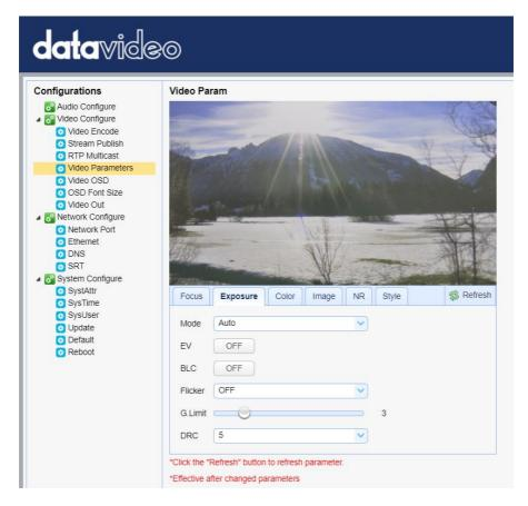
Mode: Available focus modes are Auto, Manual, SAE (Shutter Automatic Exposure), AAE (Aperture Automatic Exposure) and Bright.
