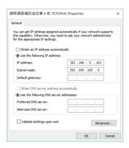
Step 10. After that, the PTC-140T and your PC are in the Static IP mode. Please open the PTC-140T web UI by using the IP address 192.168.5.163.
