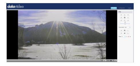
At the bottom right corner of the camera image display window, click the "Stream" button to switch between Main Stream and Sub Stream previews. See *Video Encode* in *Configuration* tab for stream settings.
