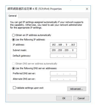
Step 10. After that, the PTC-140T and your PC are in the Static IP mode. Please open the PTC-140T web UI by using the IP address 192.168.5.163.
