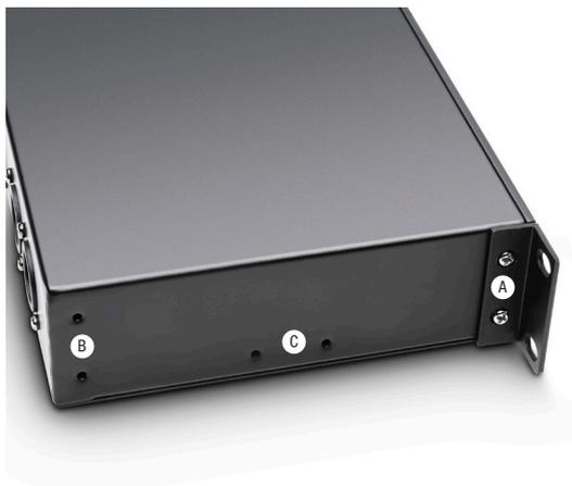
**EN** For an individual rack mounting, the rack-mounting brackets can be mounted both to the front (A), as well as to the rear (B) of the device. Wall mounting, or under table mounting is possible using the thread in the middle of the housing side (C). Only use the original screws to fasten the rack mount bracket.
